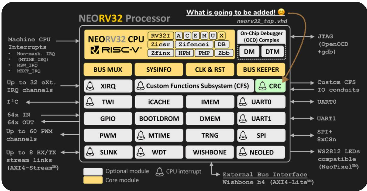
The NEORV32 processor with its NEORV32 CPU core, bus infrastructure, and comprehensive peripheral set. Our CRC32 module integrates through the Custom Functions Subsystem (CFS).
