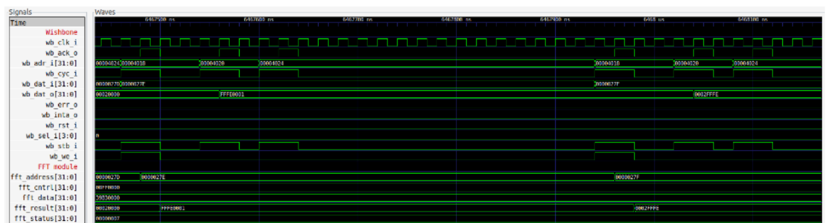
Figure A.3.: Waveform of two typical write cycles on the Wishbone bus (from FFT ROM to memory)
